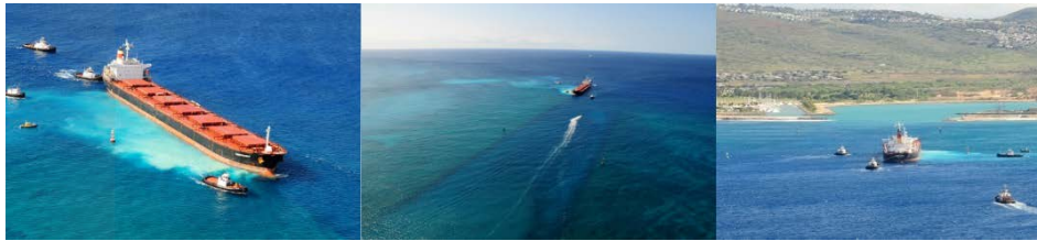
Figure 3. Aerial photos showing the Vogetrader hard aground on near shore coral reef habitat along the edge of the entrance channel. The areas of light colored water adjacent to the ship represent suspended reef material that has been crushed and turned into powder by the vessel hull. The Vogetrader (renamed the Denak Trader in 2012) is a bulk carrier that is 734 ft. (224 m) long with a beam of 104 ft. (32 m) and a draft of 39 ft. (12 m) deep. The vessel was laden with 27,000 metric tons of bulk cement powder (USCG incident report) when it ran aground.
